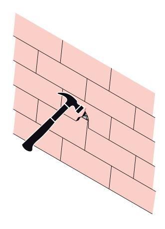
Cladding tile can be removed with push against the clip. Remaining fragments must be removed totally.
