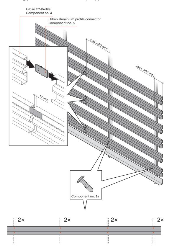
Stick two Urban T Clip per cladding tile in Urban TC profile. The rear side nose of the cladding tile must be pushed into the TC profile. The sides of the tiles should not touch.
