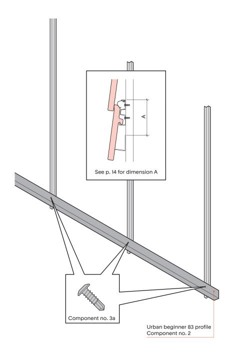
3. Affix the Omega support battens at a regular spacing.
