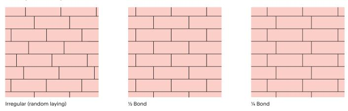
**Recommendation:** Random laying is the most installer-friendly method by far and creates less waste. The length tolerances of the tiles may be up to +/- 10 mm.
