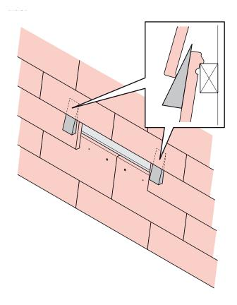
4. In the case of the Urban U-type, the hanging lug must be reduced to 5 mm.
